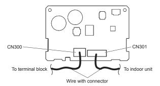
Connection depends on the PCB type of the indoor unit.
