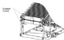
Completed Step 14b View Horizontal Left Coil Assembly
