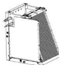
Completed Step 14b View Horizontal Left Coil Assembly
