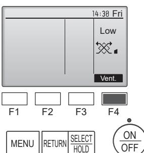
Press the [F4] button to go through the ventilation setting options in the order of "Off", "Low", and "High".
