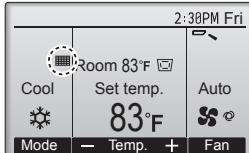
will appear on the Main display in the Full mode when it is time to clean the filters.
