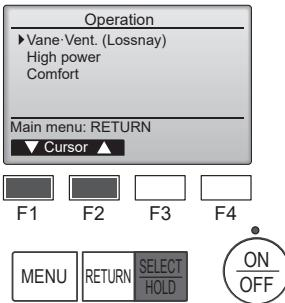
Select "Vane·Vent. (Lossnay)" from the Operation menu, and press the [SELECT/HOLD] button.
