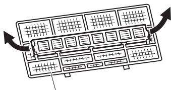
Pull to remove from the air filter
