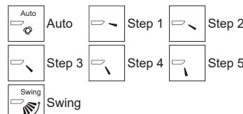
Select "Swing" to move the vanes up and down automatically. When set to "Step 1" through "Step 5", the vane will be fixed at the selected angle.
