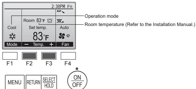
Press the [F2] button to decrease the preset temperature, and press the [F3] button to increase.
