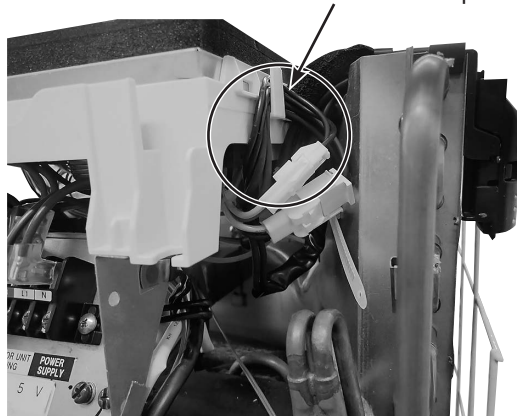
Lead wires of the defrost heater and the heater protector
