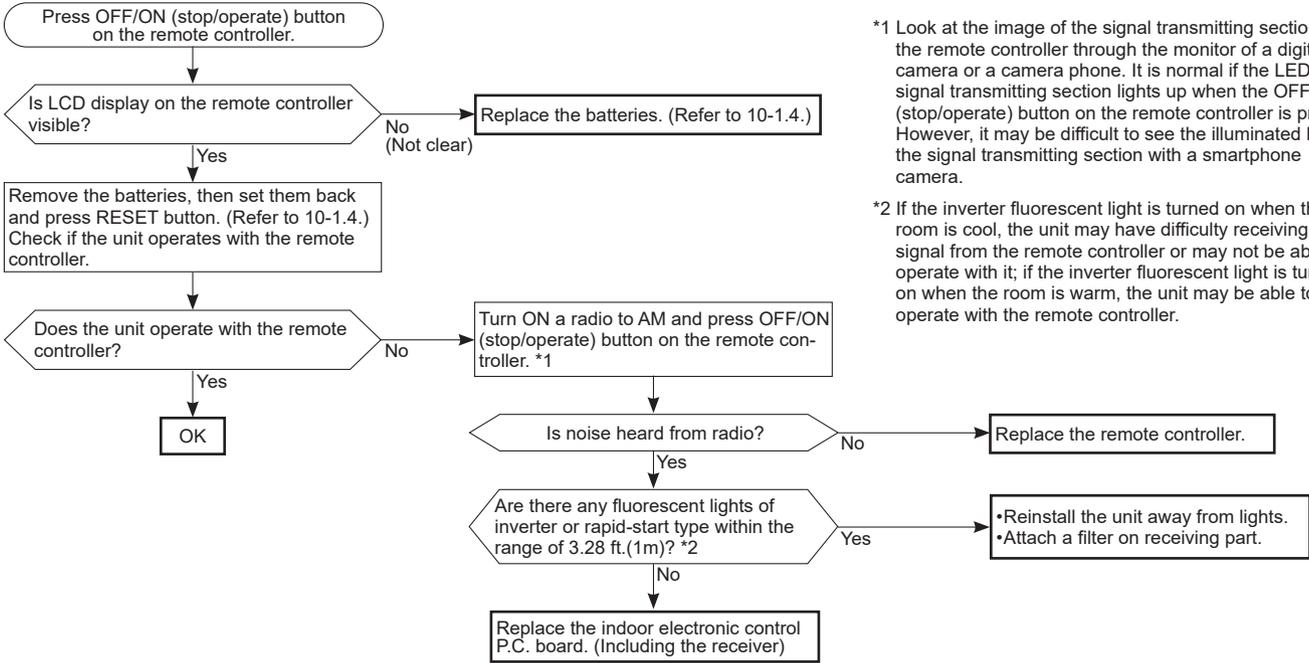
\*1 Look at the image of the signal transmitting section of the remote controller through the monitor of a digital camera or a camera phone. It is normal if the LED of the signal transmitting section lights up when the OFF/ON (stop/operate) button on the remote controller is pressed. However, it may be difficult to see the illuminated LED of the signal transmitting section with a smartphone camera.
