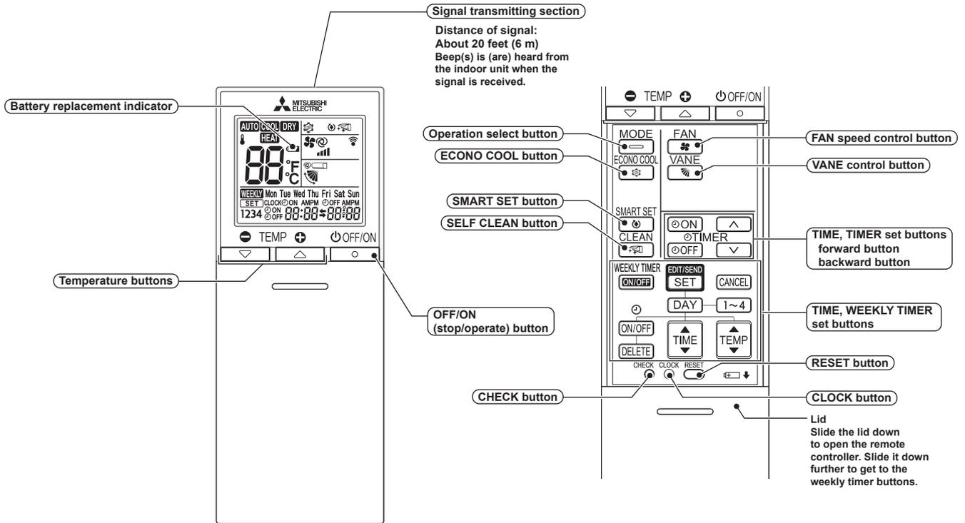
\* The backlight turns on when using the remote controller.
