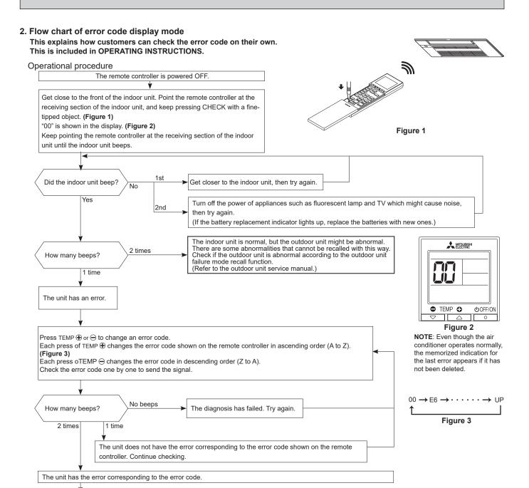
Refer to the error code on the table of indoor unit failure mode recall function (10-2.3.) or the table of outdoor unit fail-
