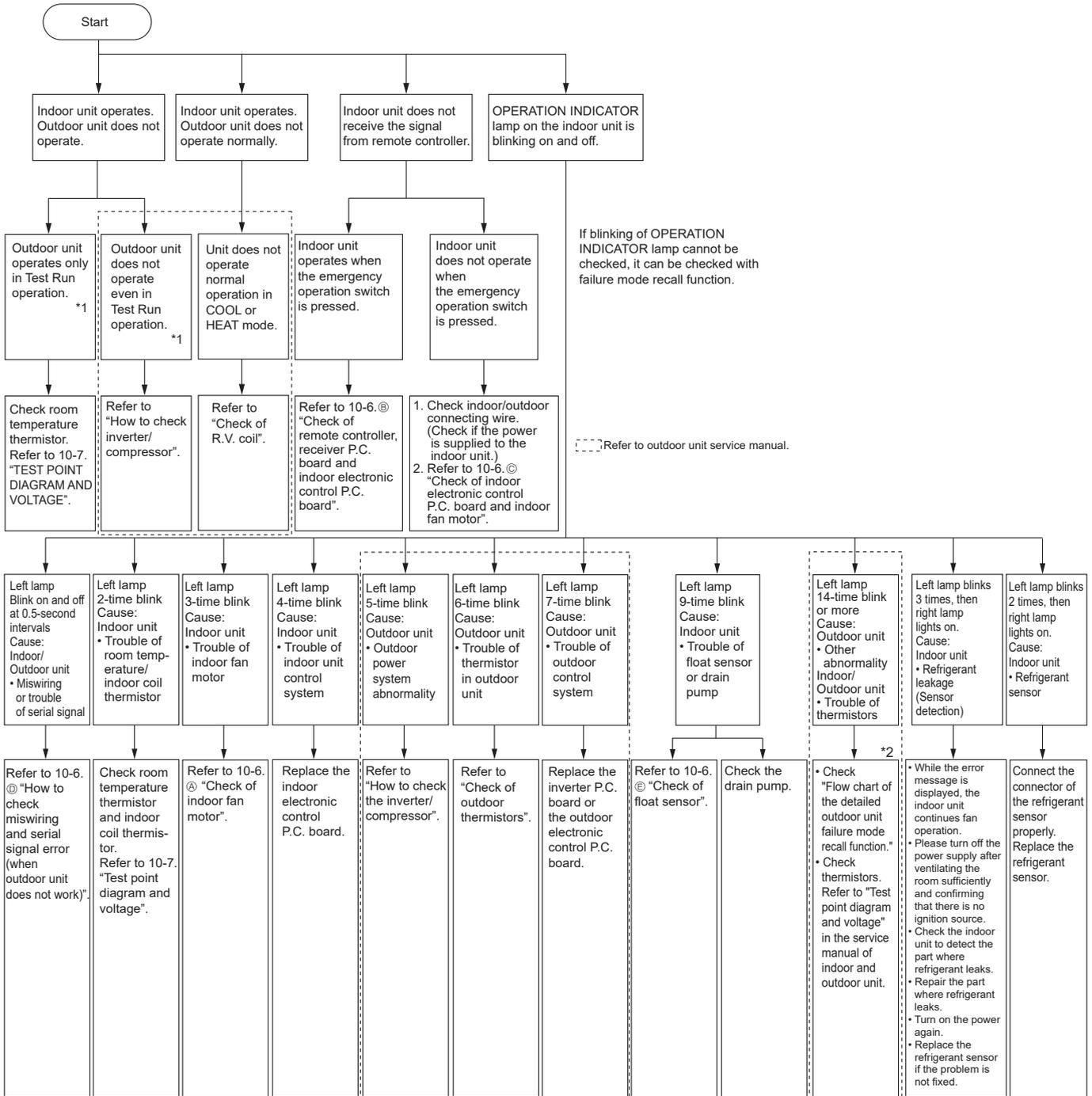
\*1 "Test Run operation" means the operation within 30 minutes after the emergency operation switch is pressed.
