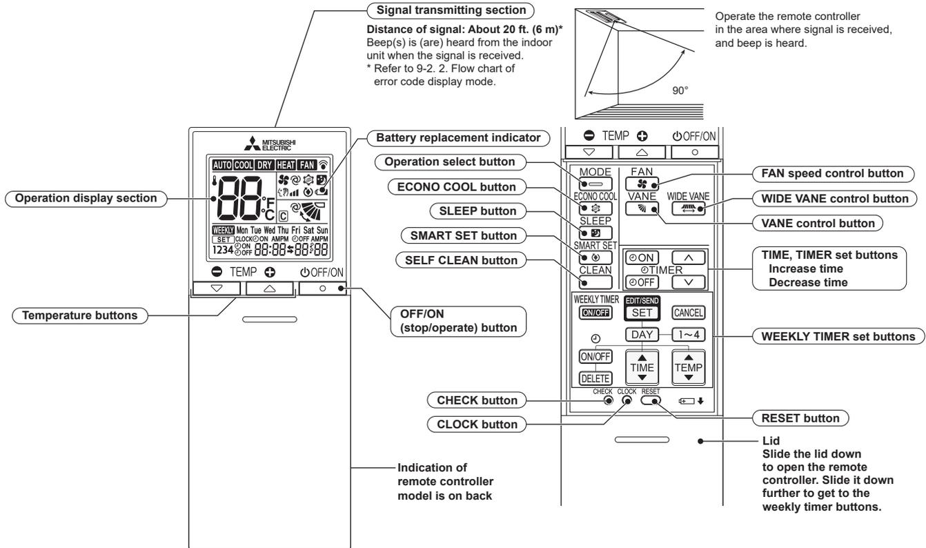
**NOTE:** Last setting will be stored after the unit is turned OFF with the remote controller. Indoor unit receives the signal of the remote controller with beeps.
