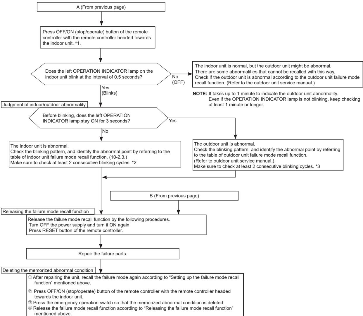
**NOTE:** It takes up to 1 minute to indicate the outdoor unit abnormality. Even if the OPERATION INDICATOR lamp is not blinking, keep checking at least 1 minute or longer.
