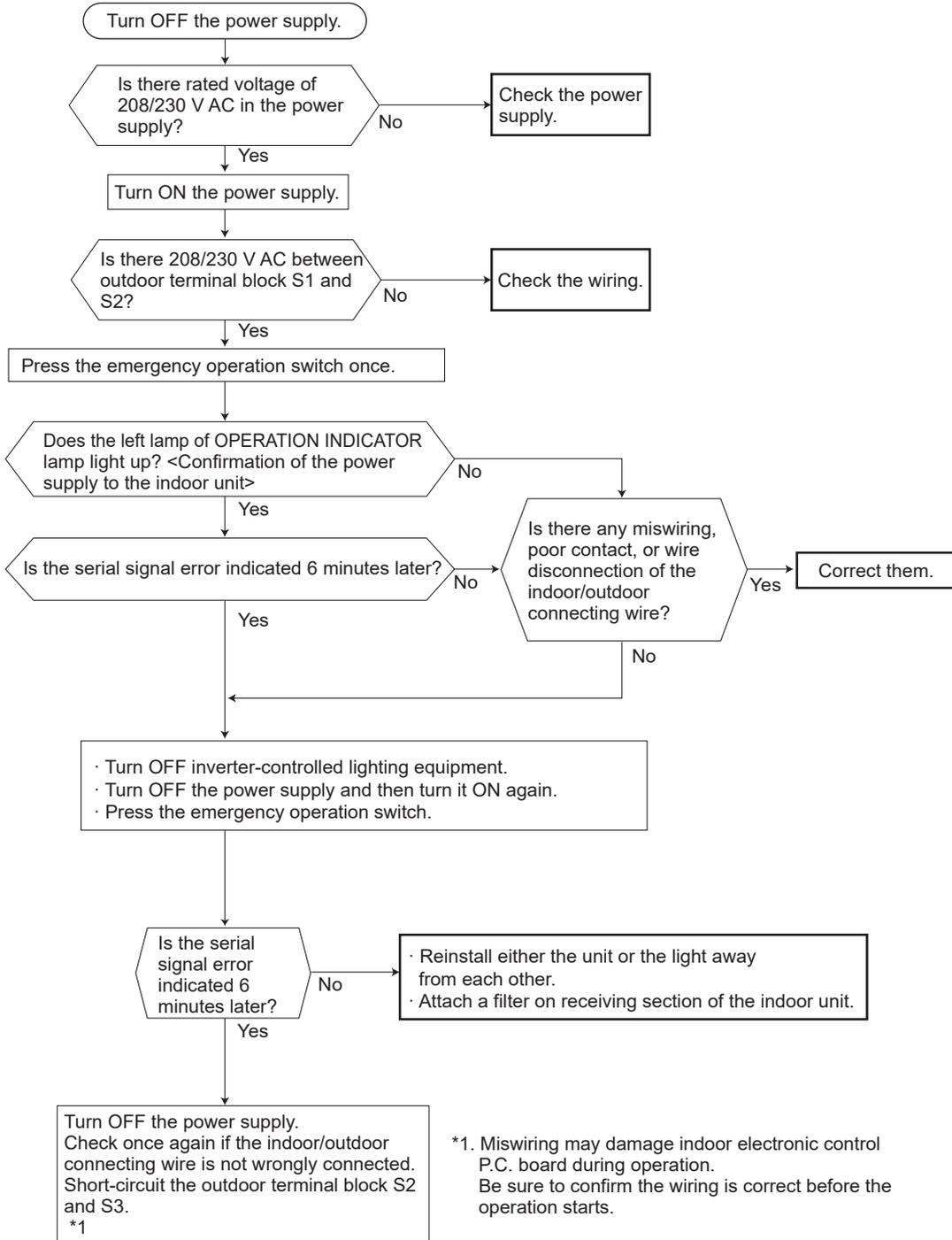
\*1. Miswiring may damage indoor electronic control P.C. board during operation. Be sure to confirm the wiring is correct before the operation starts.
