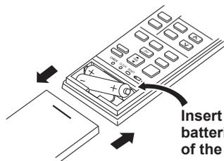
Insert the negative pole of the batteries first. Check if the polarity of the batteries is correct.
