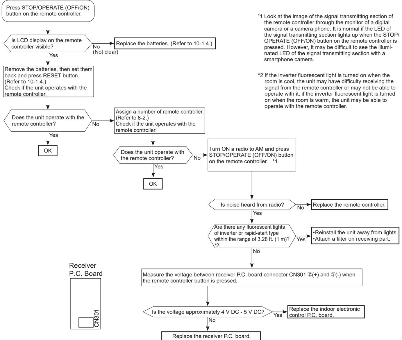
The unit cannot be operated with the remote controller.
