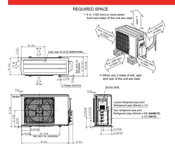
Drain hole Ø1-5/16 (KA09/12/15NAH)
