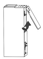
**STEP 2:** Remove the knock-out hole of the upper cover.
