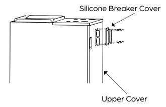
**STEP 8.** After installing the electric auxiliary heat module, apply the circuit breaker label included near the silicone breaker cover that was just installed for future reference.
