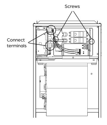
**STEP 6:** Connect the wiring according to the wiring diagram on page 10 and 11. Attach the wiring diagram sticker provided to the inside of the front cover for future reference.
