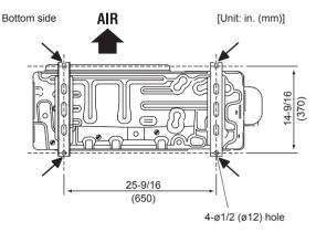
Fix securely with bolts on a solid block. (Use 4 sets of commercially available M10 bolt, nut and washer.)
