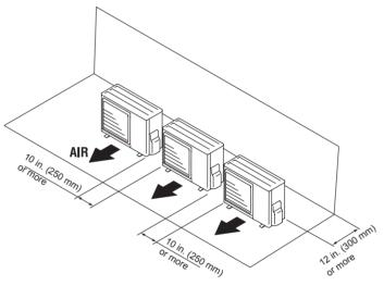
No more than 3 units must be installed side by side.
