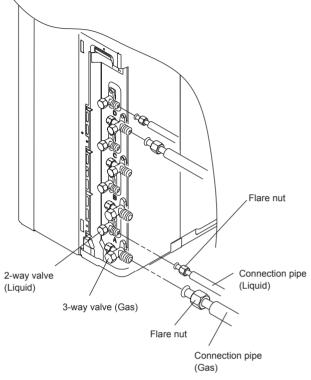
(4) When the flare nut is tightened properly by your hand, use a torque wrench to finally tighten it.
