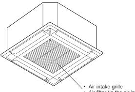
Air filter (in the air intake grille)
