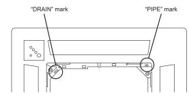
· Align the stamped marks on the cassette grille to the pipe and the drain of the indoor unit.
