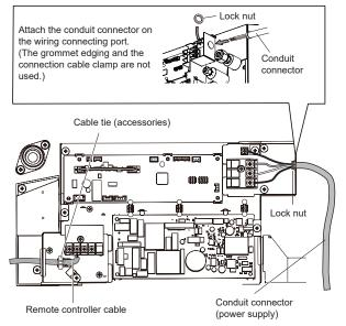
Do not bind the connection cable (power supply) and other cables together.
