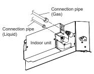
(3) When the flare nut is tightened properly by your hand, hold the body side coupling with a wrench, then tighten with a torque wrench. (Refer to the following table for the flare nut tightening torques.)
