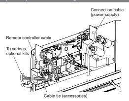
Do not bind the connection cable (power supply) and other cables together.
