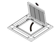
4.2. Installing the panel to indoor unit
