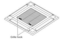
(2) Open the intake grille and remove.
