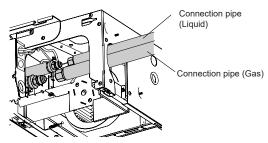
(3) When the flare nut is tightened properly by your hand, hold the body side coupling with a separate spanner, then tighten with a torque wrench. (See the table below for the flare nut tightening torques.)
