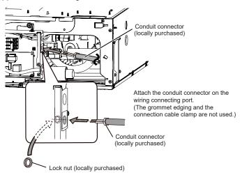
(3) Pass the remote controller cable through the hole ,and fix the cable with the cable tie.
