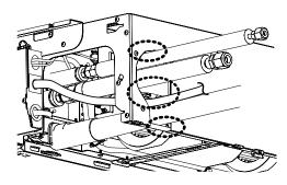
(2) Align three hooks of the side panel, and fix it to the backward. Then, fix it with the screw.
