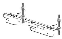
(3) Attach the unit body to the fixed suspension fittings, tighten two bolts on each side.
