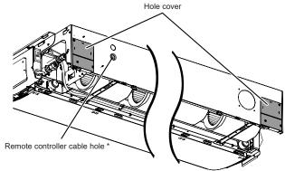
\* When using a wired remote control, please pass through the remote controller cable hole.
