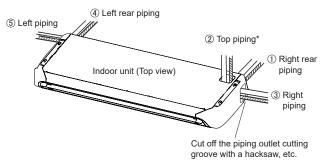
\* ②, A Drain pump unit (Optional parts) and an Auxiliary pipe assembly (Optional parts) are required.
