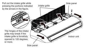
Removing the casing guard
