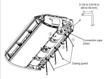
Finally, fix two positions using the screw removed in the previous step and the accessory self-tapping screw.
