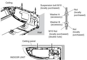
(2) Fasten the indoor unit into place by tightening-up the bolts and the M10 nuts. Make sure that unit is secure and will not shift back and forth.
