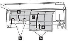
2 Remove dust by using a vacuum cleaner or by washing the filter. When you wash the filter, use neutral household detergent and warm water.
